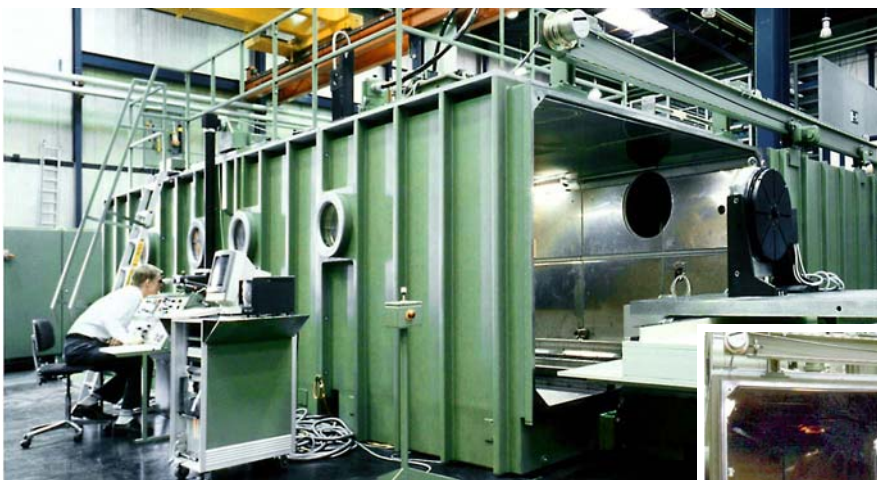
EB Großkammermaschine EBOCAM KS 440 – G 300 KM
